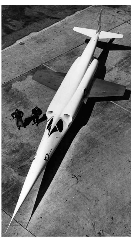
In this 1953 photo taken at Edwards AFB, Calif., admirers ogle the one and only X-3, an experimental aircraft built by Douglas Aircraft. The futuristic, needle-nosed craft—dubbed "Stiletto"—was created to test aircraft at sustained supersonic flight, but it was underpowered and could not exceed Mach 1. USAF turned it over to the National Advisory Committee for Aeronautics, which retired it in 1956. ■
